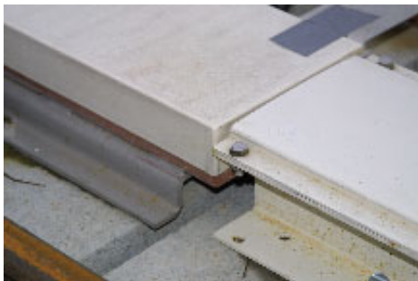
Fig. 3 Change from long-stator(left) to short-stator motor (reaction plate at right)
