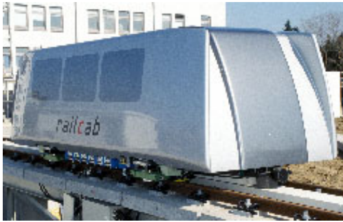
Fig. 2 Shuttle of NBP test track
